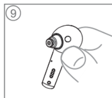
5. Insert the new wax guard into the opening of the sound outlet and press it gently, and pull the holder straight out.
