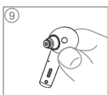
5. Insert the new wax guard into the opening of the sound outlet and press it gently, and pull the holder straight out.
